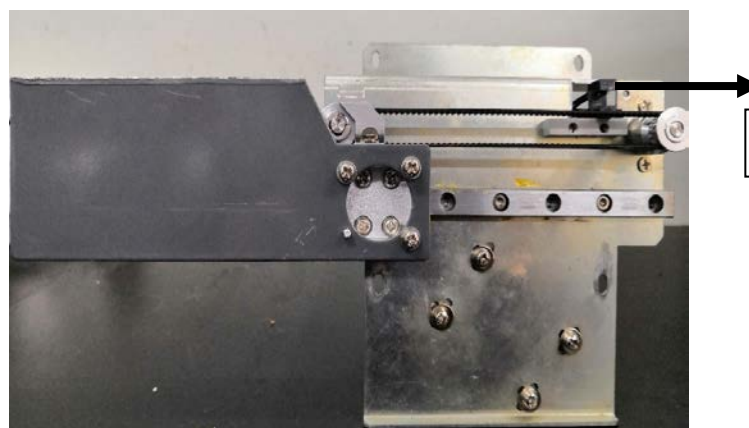
2-5-3 opening/closing door assembly
