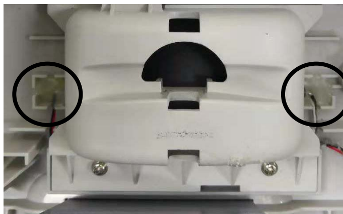
2-6-2 left-right bijection optocoupler
