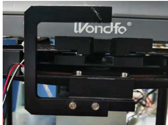
2-6-1 U-type bijection optocoupler
